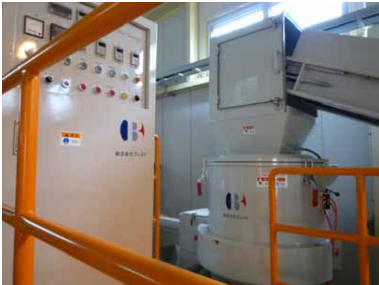
Granulator of the Plastic Film
