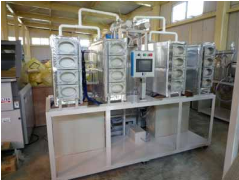
Granulator of the Plastic Film
