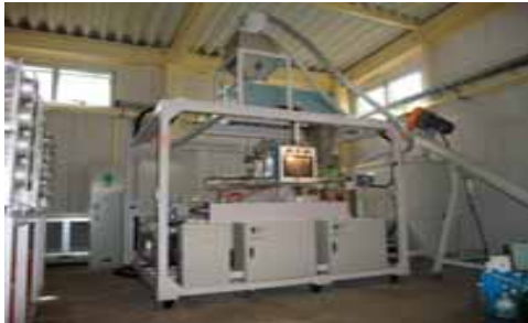
Plastic to Oil Machine: B 2 4 0 ( 10Kg/Hr )
