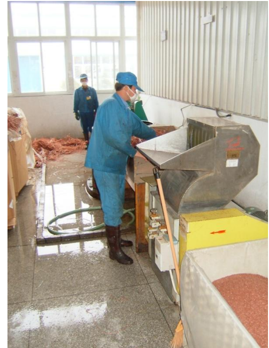
Nagget system to separate copper and plastics. (Dec, 2004)
